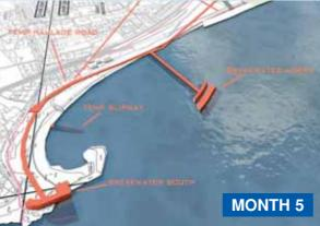
Temporary Causeway complete. New Wall laid at right angles to it. Also new wall laid to seaward of old East Wall.
